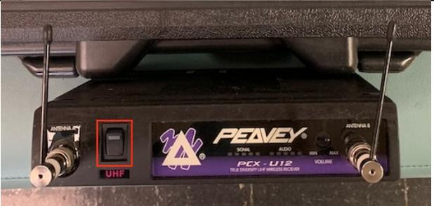
A close-up photograph of the front panel of a Peavey PCX-U12 wireless receiver. The power switch, located on the left side of the panel, is highlighted with a red rectangular box. The panel also features two antennas, a volume knob, and various input ports.                                                                           |
