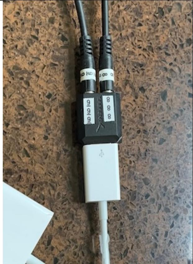
10. Plug the end of the audio cable with the **(0)** label into the Harbinger speaker Input 2 jack with the matching **(0)** label. This cable supplies the computer audio to the in-room speakers. The cable should be in the computer bag pouch, and will have a **GREEN** tag. The other end of this cable should be connected to the computer USB audio adapter. (NOTE: There are extender cables available in the **MAIN SPEAKER** bag if the cable is too short. They will have **BLUE** tags.)
