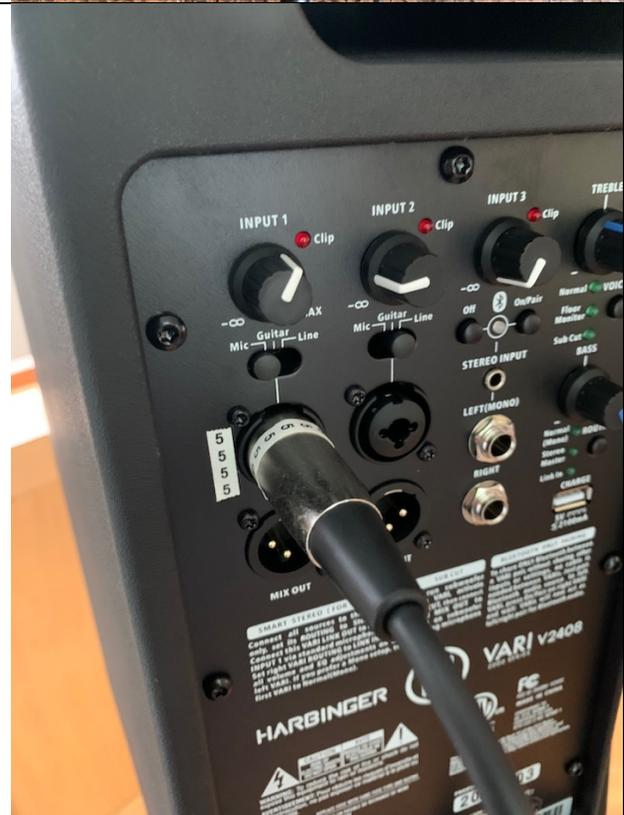
6. Connect the end of the short audio cable with the **(6)** label to the audio output jack on the Peavey wireless microphone unit with the matching **(6)** label. Note that the 6 has a line underneath it so you don't confuse it with a 9. This carries the audio from the Peavey wireless microphone unit to the Harbinger Speaker Input 1 jack. This cable should be found in the Peavey wireless microphone case, and will have a **WHITE** tag.
