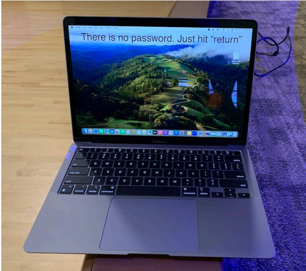
The MacBook Air is a standard laptop computer, with a display, keyboard and trackpad. The power button is the unlabeled button in the top right corner of the keyboard, just to the right of the F12 key, and just above the Delete key. (See page 18) The function keys have special functions as noted by the symbols above their function numbers.
