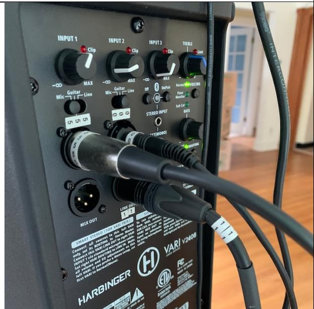
12. Plug the end of the long audio cable with the **(12)** label into the **INPUT 1** jack on the **SECOND SPEAKER** with the matching **(12)** label. The long audio cable is stored in the second speaker bag and has a RED tag.
