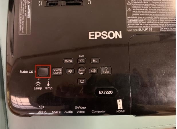
A close-up photograph of the control panel of an Epson projector. The power button, located next to the 'Status CB' indicator and above the 'Lamp' and 'Temp' indicators, is highlighted with a red rectangular box. Other buttons include 'Menu', 'H/V', 'Esc', 'Source Search', 'Enter', and 'Help'. The model number 'EX7220' is visible. |
