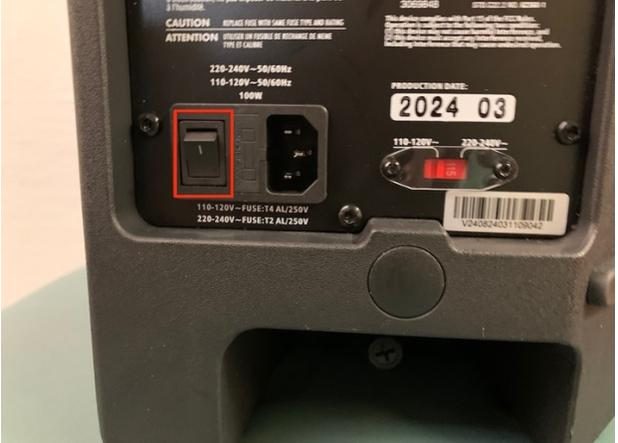
A close-up photograph of the back panel of a Harbinger speaker. The power switch, located in the lower left corner next to the power cord input, is highlighted with a red rectangular box. The panel includes technical specifications such as '220-240V-50/60Hz 110-120V-50/60Hz 100W' and a production date of '2024 03'.                |
