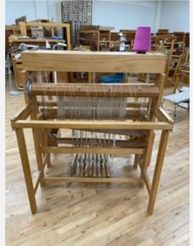
6. Move back beam from castle storage to back and secure with pins
