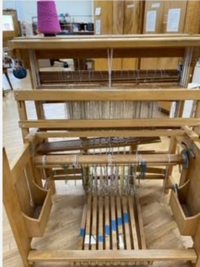
3. Drop cloth beam and pin in place with cotter pins
