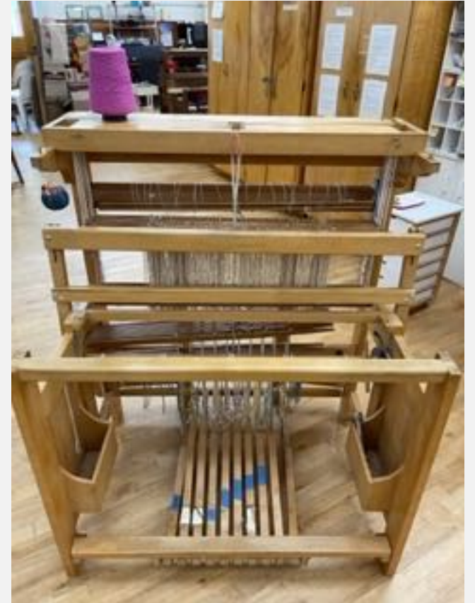
4. Move breast beam from castle storage to front of loom
